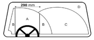
Zone A Damage up to 10mm | Zone C Damage up to 25mm Zone B Damage up to 15mm | Zone D Damage up to 40mm
